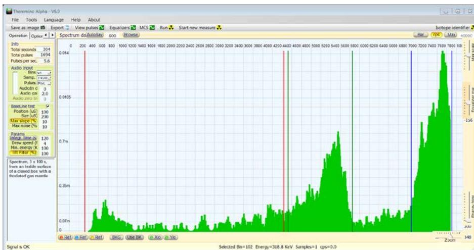
**Fig. 5.** Bi-212 (6.0 MeV) and Po-212 (8.7 MeV) from an inside surface of a box, closed for several days, with a thoriated gas mantle, measured 3 x 100 s.
