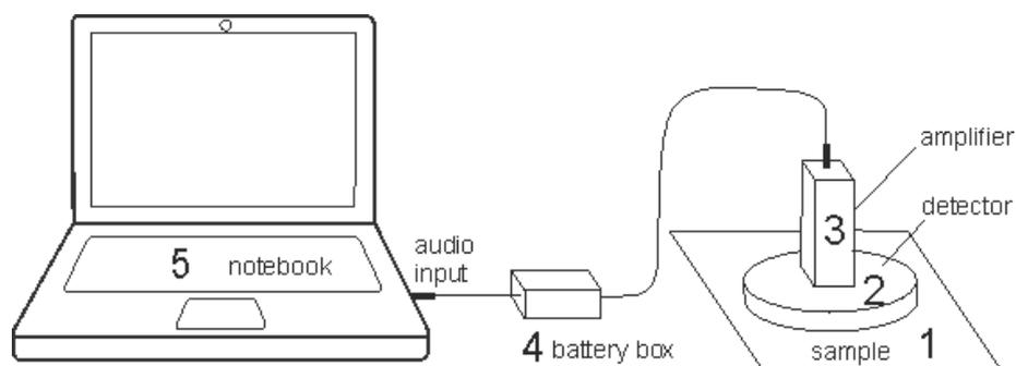
**Fig. 1.** Scheme of the spectrometer. The silicon alpha detector (2) is placed on top of the sample (1). A homebuilt pulse amplifier (3) is directly attached to the detector. A battery (4) supplies the amplifier. Pulses are fed into the audio input of the computer (5) running the pulse height analyzer software.
