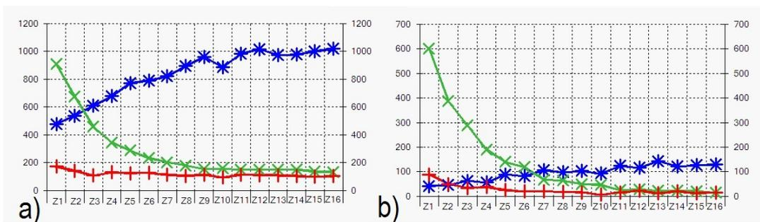
**Fig. 7.** Count rates vs time (16 x 100 s) for Po-218 (green) and Po-214 (blue), collected as in Fig 4 from indoor air (a) and from outdoor air (b). Note the significant difference of the blue curves (Po-214), due to the factor of equilibrium which is high for indoor air and low for outdoor air.
