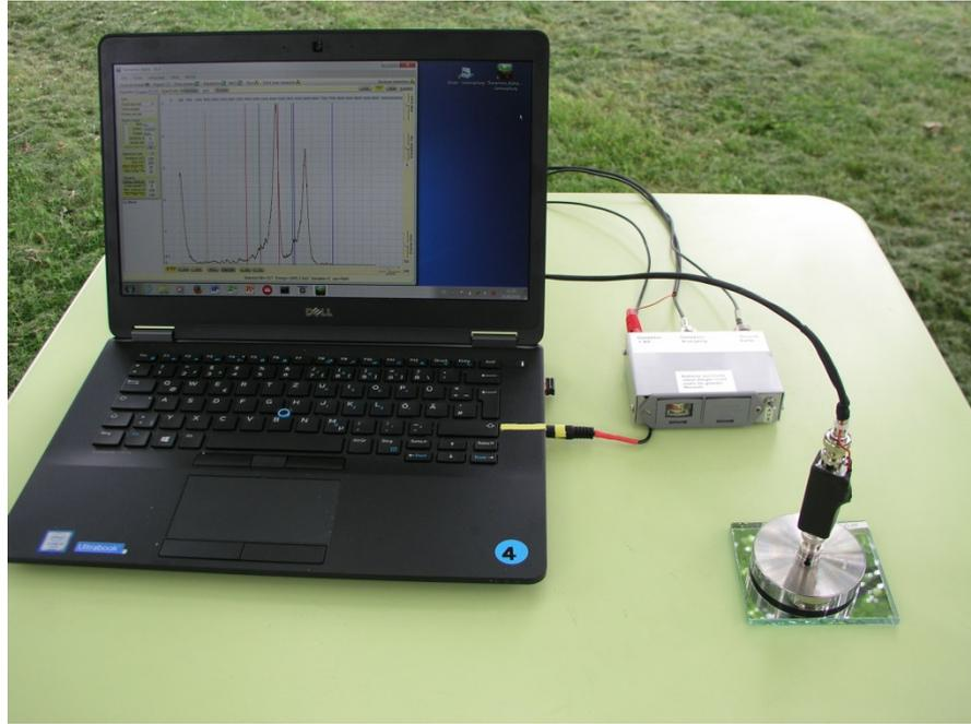
**Fig. 2.** Photo of the complete spectrometer. The detector (2) is a Canberra CAM-2000-AB.
