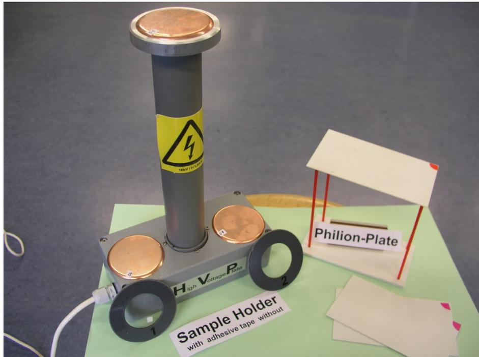
**Fig. 3.** Two instruments to collect airborne positively charged radon and thoron decay products. Left: Electrostatic sampler. The base contains a mains driven -14 kV high voltage generator which connects to a 6 cm diameter copper plate on top of an insulating tower 30 cm above the surface on which the base is standing. Right: Philion-Plate, polystyrene, simply charged to -20 kV by forceful rubbing for 60 s with the sharp edge of a piece of wood.
