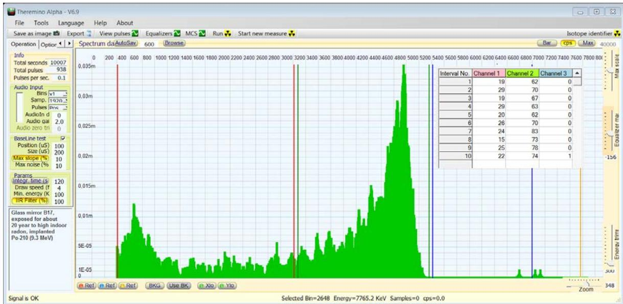
**Fig. 4.** Spectrum of a glass mirror front surface, exposed for about 20 years to high indoor radon. Ortec detector 12 cm<sup>2</sup>, efficiency 40 %, background (Cu) 6 counts per 1000 s. The energy ranges are explained by the insert of fig. 6. Sample with Po-210 (5.3 MeV, misspelled 9.3) yields 70 counts per 1000 s, equivalent to 130 Bq m<sup>-2</sup> and about 5.2 kBq m<sup>-3</sup> Rn-222. The pulses on the left are from beta emitters.
