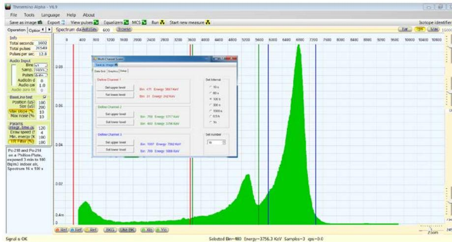
**Fig. 6.** Energy spectrum of Po-218 (6.0 MeV) and Po-214 (7.7 MeV), collected on a Philion-Plate, exposed for 3 min to indoor air with about 100 Bq m<sup>-3</sup> Rn-222 and measured for 16 x 100 s. The vertical lines in red, green and blue define the spectral windows and can be set by mouse click. See also Fig. 7a.
