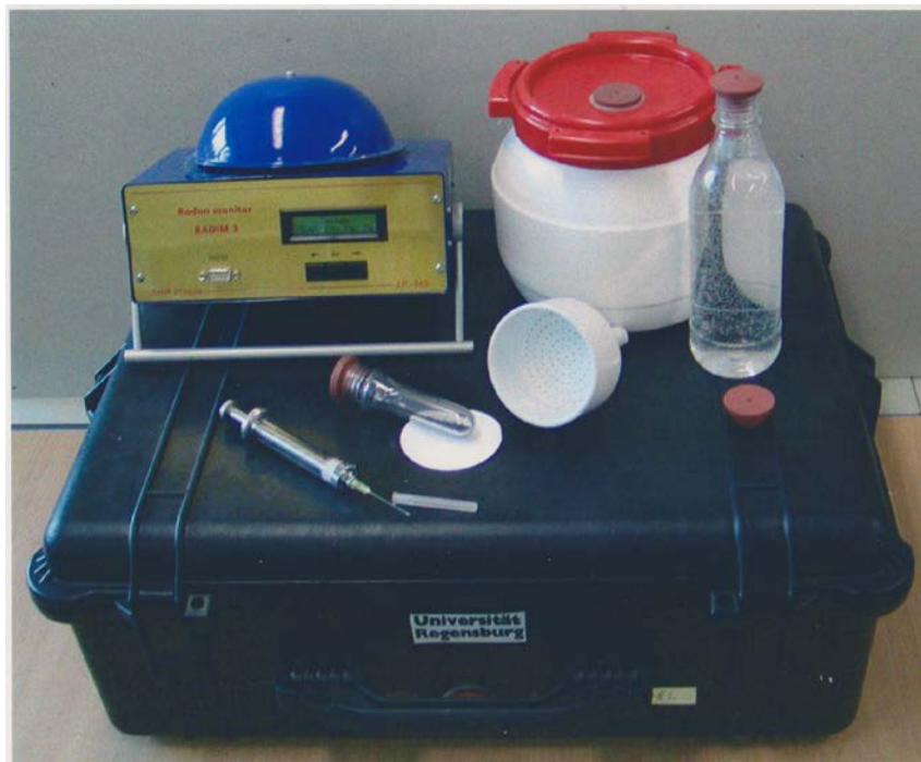
Fig. 4: The parts for in-laboratory calibration of Rn monitors
