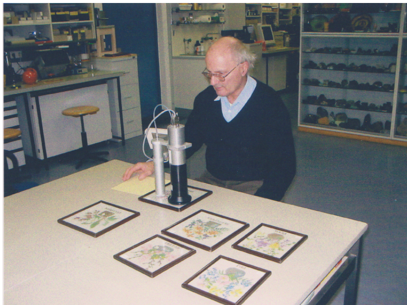
Fig. 5: The portable large-area alpha detector in the author's laboratory
