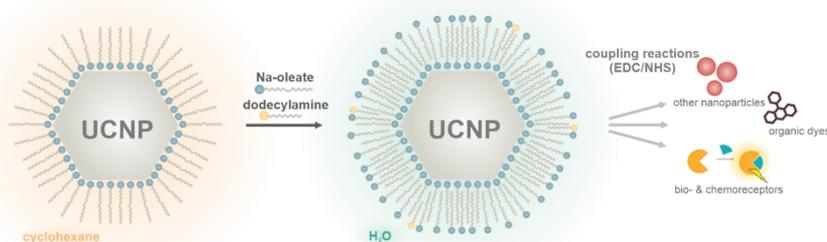
bright bilayer-modified particles have been functionalized with organic dyes, without losing colloidal stability, suitable for FRET applications intended for singlet oxygen detection and for sensing of reactive oxygen species.
